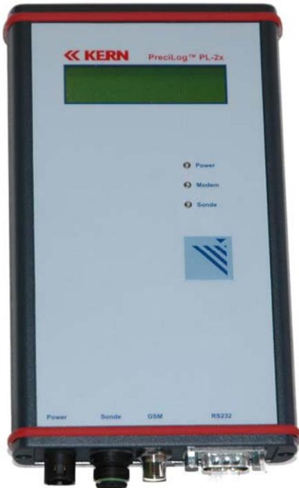
An extra small and robust datalogger for automated storage of waterlevel, temperature and other values with analog or digital interface (DeltaFlex, KS-3).
